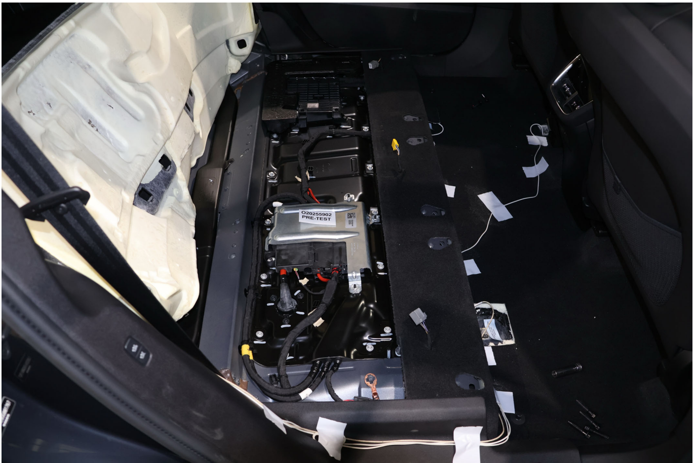
Photo No. 305-09 - Pre-Impact View of Propulsion Battery
